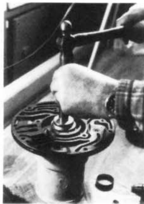
INSTALLING OIL PUMP BUSHING
