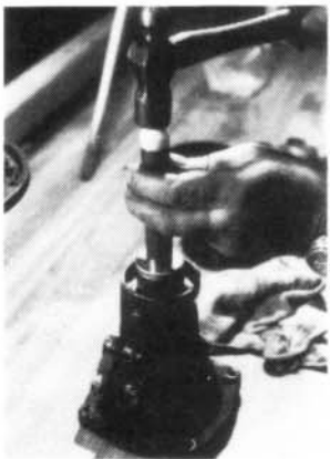
INSTALLING EXTENSION HOUSING BUSHING
