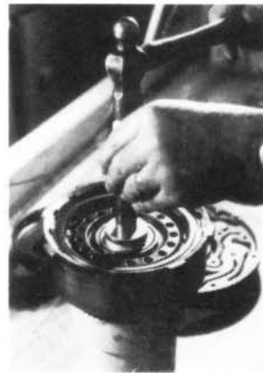
INSTALLING DIRECT CLUTCH BUSHING
