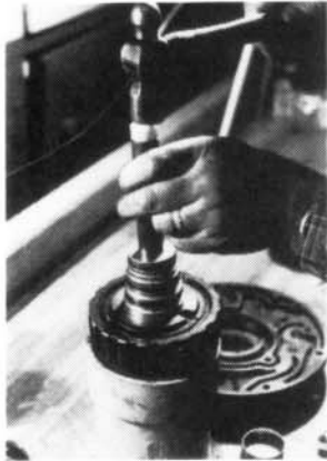
INSTALLING RING GEAR BUSHING
