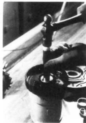
INSTALLING REACTION CARRIER BUSHING
