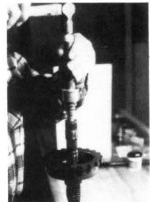
INSTALLING OUTPUT SHAFT BUSHING
